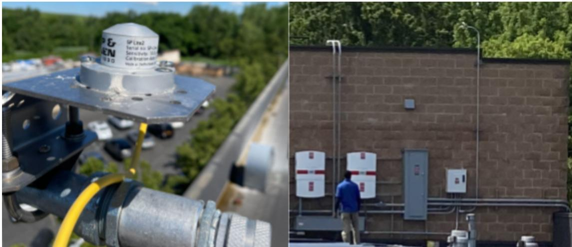
Figure 3: Staten Island UGE (Left) Pyranometer | (Right) Data Logging System
